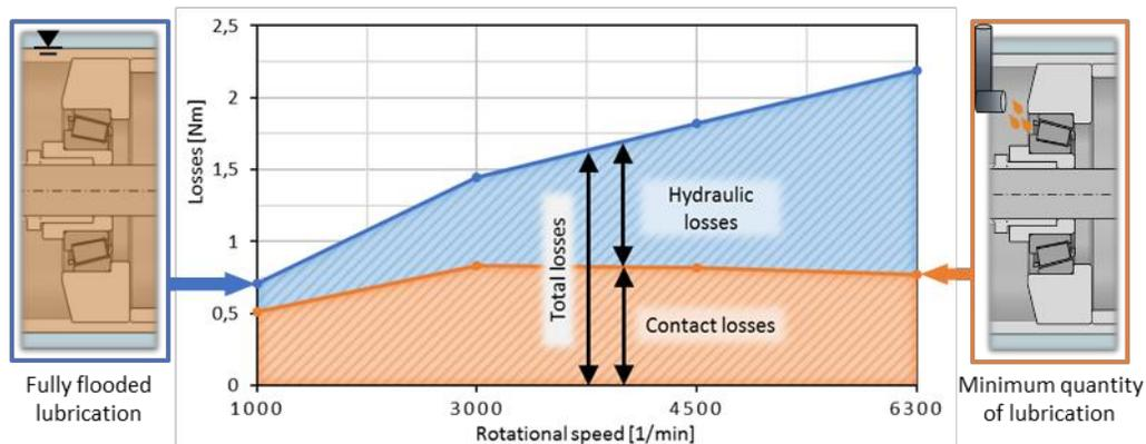
Figure 2: Example for the determination of the hydraulic losses with the variation of the oil level at a fully-flooded tapered roller bearing 32208
