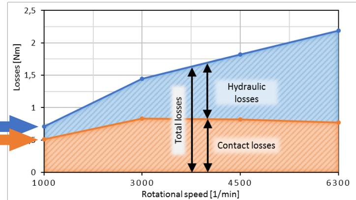
$$\text{Fully flooded lubrication} - \text{Minimum quantity of lubrication} = \text{Hydraulic losses}$$
