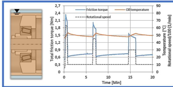
Fully flooded lubrication
