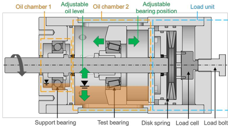
Figure 1: Test bench for the experimental investigation of hydraulic losses in horizontal bearing arrangements [2].
